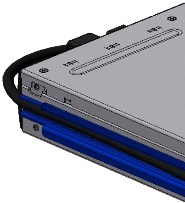
**Figure 14: Transfer Power Cord Finished**
