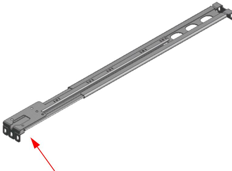
This side of the rail kit goes on the side of the rack you will slide the switch into. This is the same side of the switch that will be next to the vertical support.
