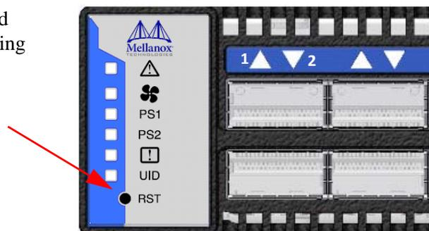
This button resets both the CPU of the switch device and the CPU of the management module. It thereby resets all of the ports by bringing them down and powering them up when the button is pushed. A quick push of this button performs this reset. When the button is held down for 15 seconds the switch is reset and the password is deleted. You will then be able to enter without a password and make a new password for the user admin.
