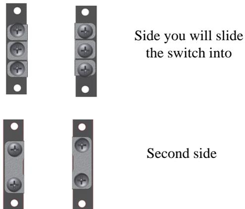
5. Clip 6 caged nuts into the holes in the rack on the side of the rack you will be sliding the switch into. Check that both sides of the switch, power side and connector side, are at the same level in the rack.
